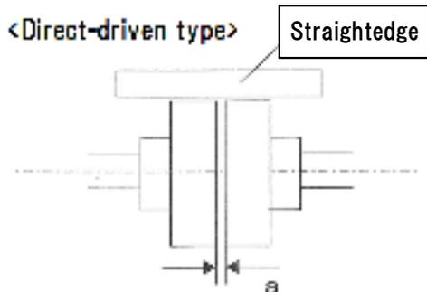
Make an adjustment with a straightedge so that the outer edges of the shaft couplings on the right and left can align with each other and clearance (a) can be uniform over the entire circumference.
