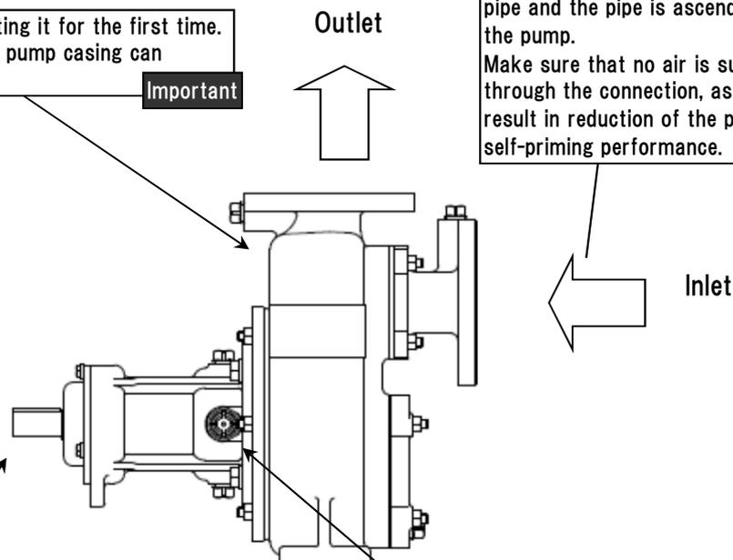
No external adjustment is required because a special mechanical seal is used for the shaft seal unit.
